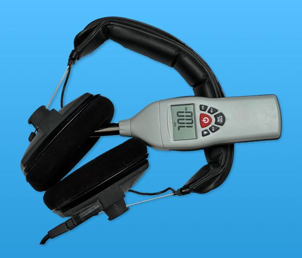
Position the calibrated dB meter with the microphone in the headphone directly facing the driver. Ensure that the dB meter is configured to measure in dBA, and consider utilizing fast response and average settings if desired.
