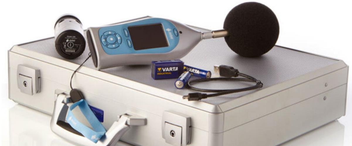
Acquire a decibel meter, also known as a sound pressure meter, capable of measuring frequencies between 125Hz and 8000Hz. For enhanced accuracy, choose a hardware meter that includes a calibration certificate. Consider selecting a meter equipped with a test tone generator for self-recalibration or arrange for periodic recalibration with the supplier. Ensure the meter measures in dBA, as HearingScan Pro can automatically convert to dB HL.
