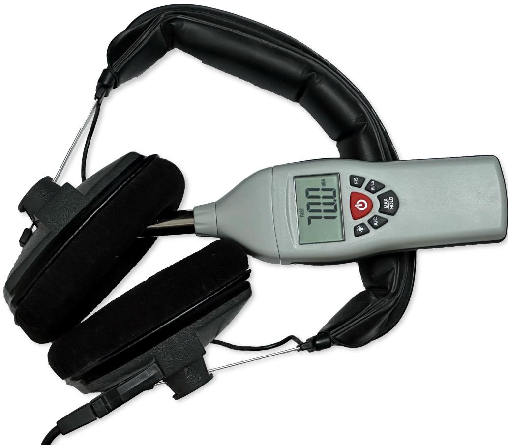
Position the dB meter directly at the location of the headphone drivers. While a 90-degree angle is preferred, larger dB meters and/or snug-fitting headphones may allow for measurements to be taken as depicted in the image. Make sure your headphone amplifier is at maximum volume and warmed up. For most amplifiers 10
